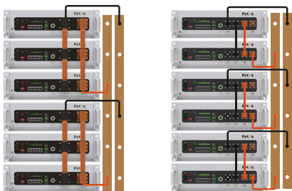
Figure 5-1 Schematic diagram of power cable connection
