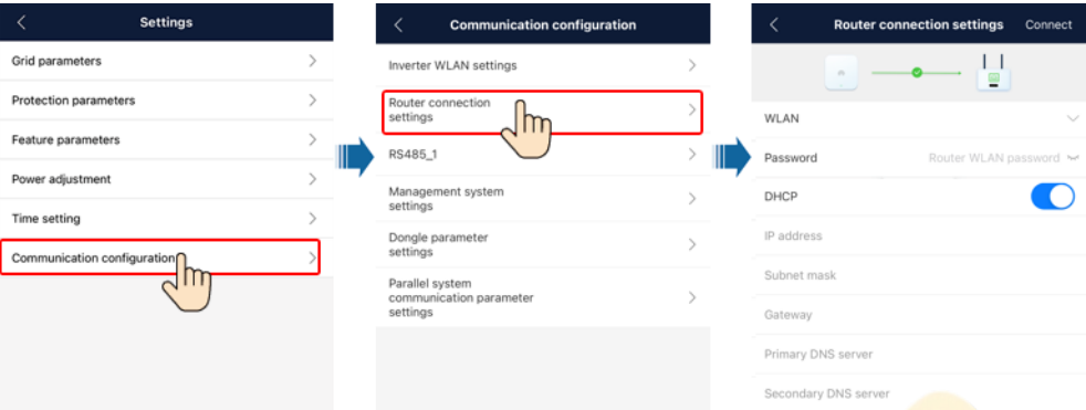
Figure 6-3 Inverter communication settings
