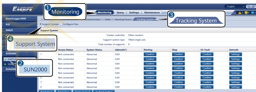
Figure 6-59 Support system (tracking system)
