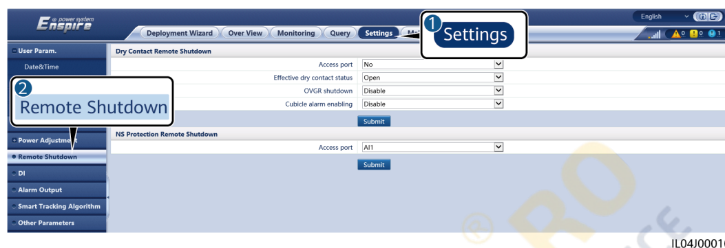
Figure 6-92 Dry contact remote shutdown
