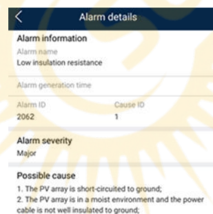
Figure E-1 Alarm details
