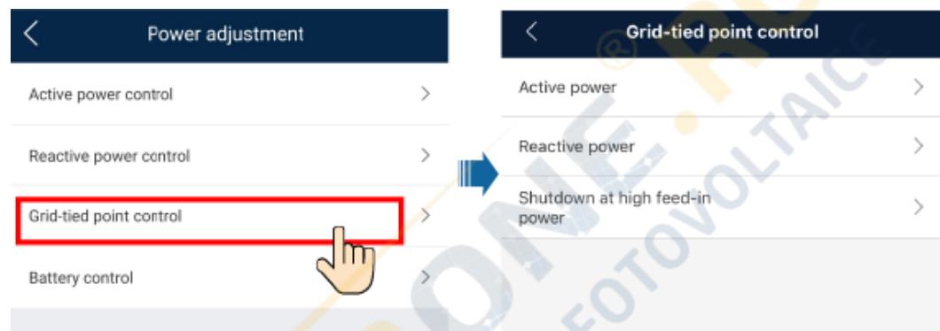
Figure 7-5 Grid-tied point control
