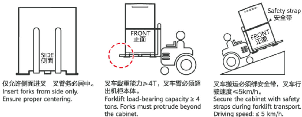
Figure 3-1 Loading and unloading requirements
